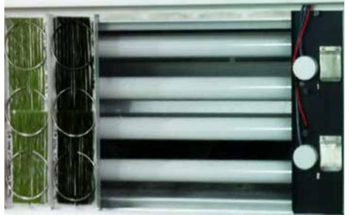
**QUV accelerated testing shows that the newest version of UltraLoc is up to 5X more stable than competitive backing systems.**
